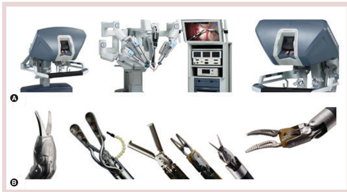
Figure 7. Surgical instruments. (A) The da Vinci Surgical System Si, (B) Endowrist instruments. © 2014 Intuitive Surgical, Inc.
