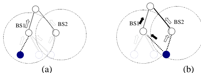
Figure 3. Smooth handoff between neighboring cells: (a) MN joins through BS1, (b) as the MN moves into BS2's covering region it joins through BS2, when it starts getting packets from BS2 it sends a leave/prune through BS1.
